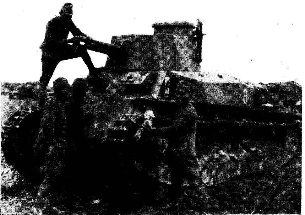
Figure 58.—Model 94 (1934) medium tank, left front. Note exterior turret machine-gun mount.
